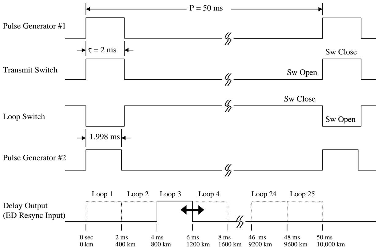
**Figure 2:** Example Circulating Loop Timing Diagram
