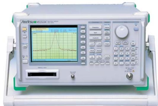
Using this multi-screen display allows two spectra with different frequencies to be displayed simultaneously. For example, this enables convenient viewing of the center frequency of interest as well as a wider or different frequency sweep at the same time.
