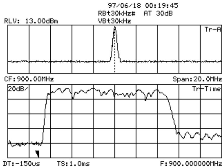
Figure 6. Split-screen frequency domain and time domain displays.
