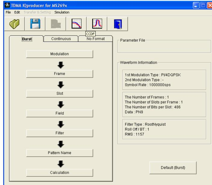
F. Select the Burst tab as RKE or TPMS signals are RF bursts of FSK frames.
