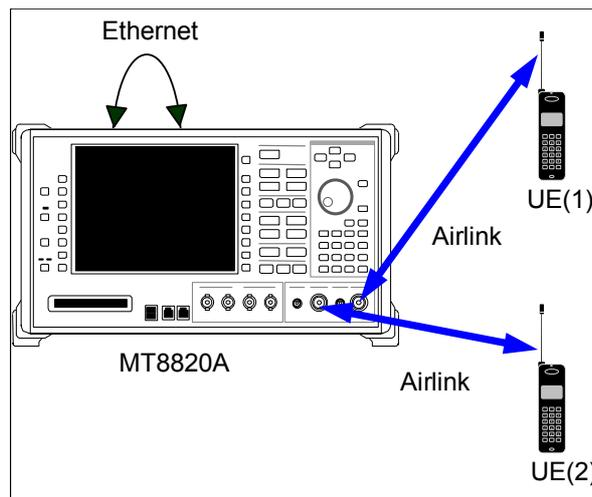
Connection for one set of MT8820A supporting parallel phone measurement
