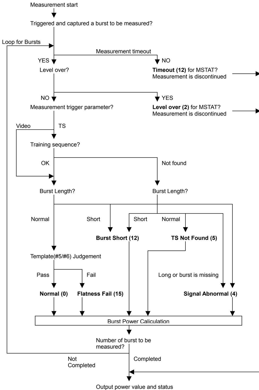
Fig. 2.8.1-2 Detection procedure of error status
