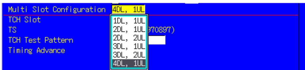
TX measurement is performed with the setting of the maximum number of slots that can be transmitted by a MS.
