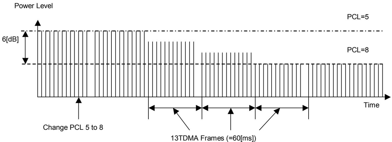
Fig. 2.13-1 Power Control by using SACCH Channel (In case of changing from PCL 5 to 8)
