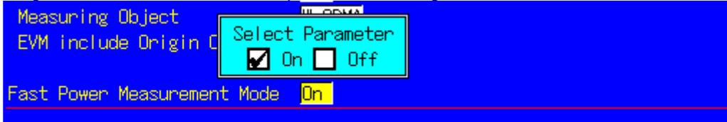
1. Execute **SCRSEL FMEAS** and display the Fundamental Measurement Screen.
