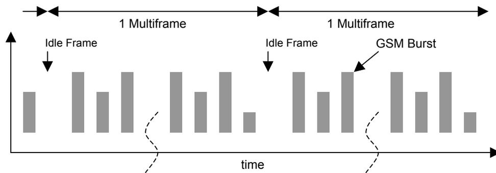
Fig. 2.8.3-1 Signal under test in Multiframe Phase Error measurement
