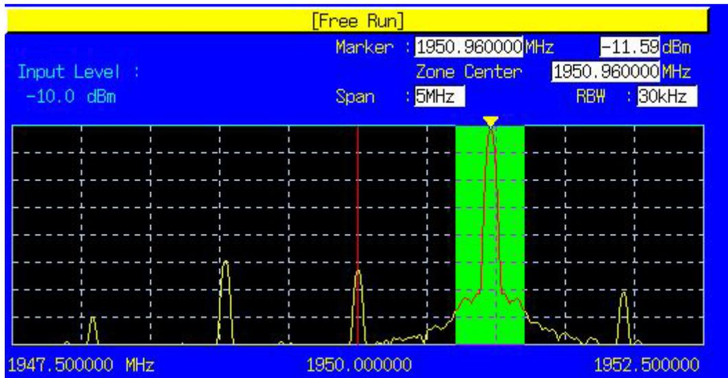
1. Execute **SCRSEL SPMON** and display the Spectrum Monitor screen.
