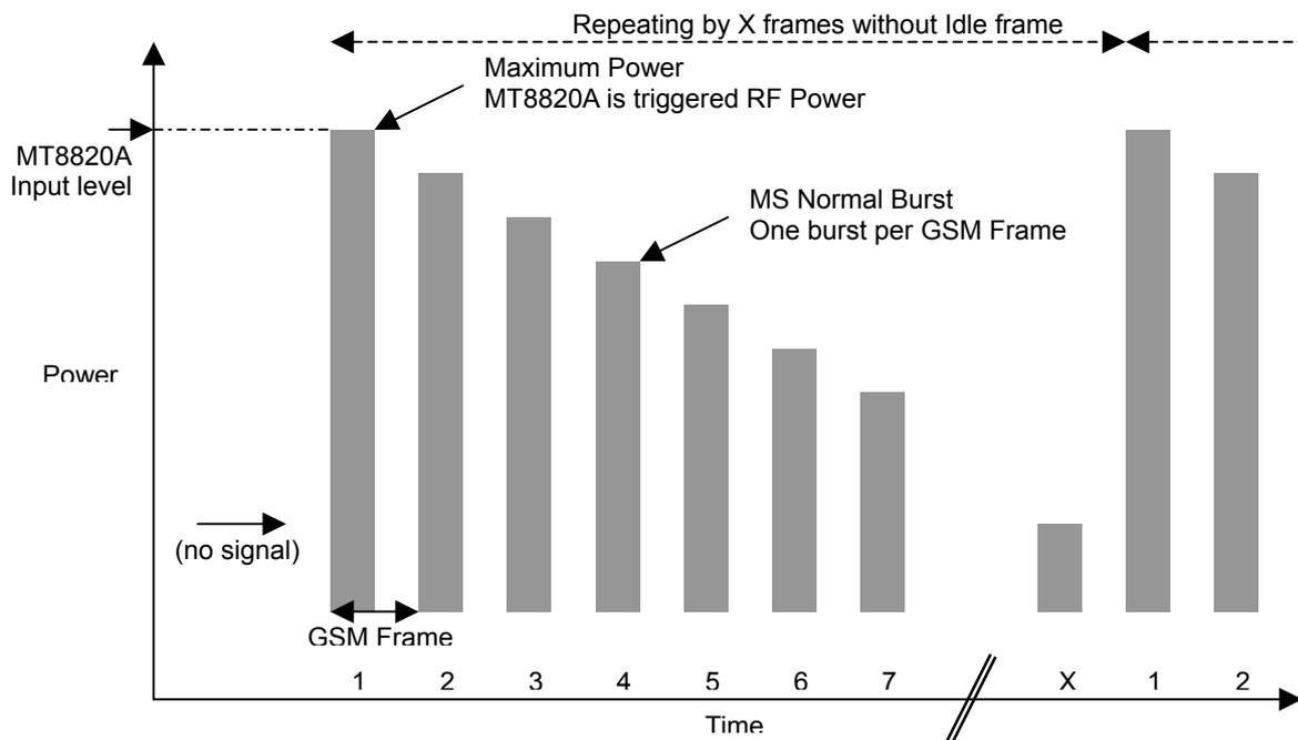
Fig.2.8.1-1 Specification of the signal under test in Multi-Burst RF Power measurement
