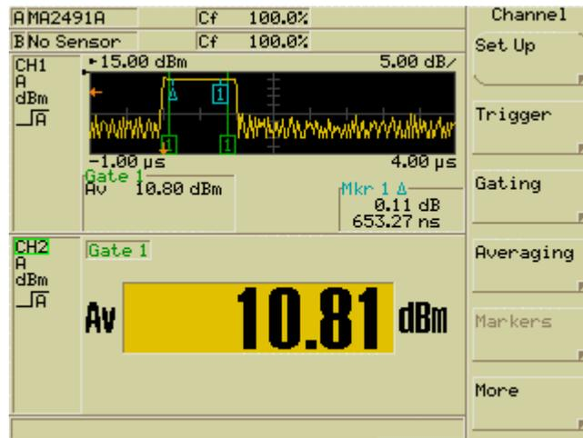
Figure 5. Dual Channel Display showing a pulse measurement
