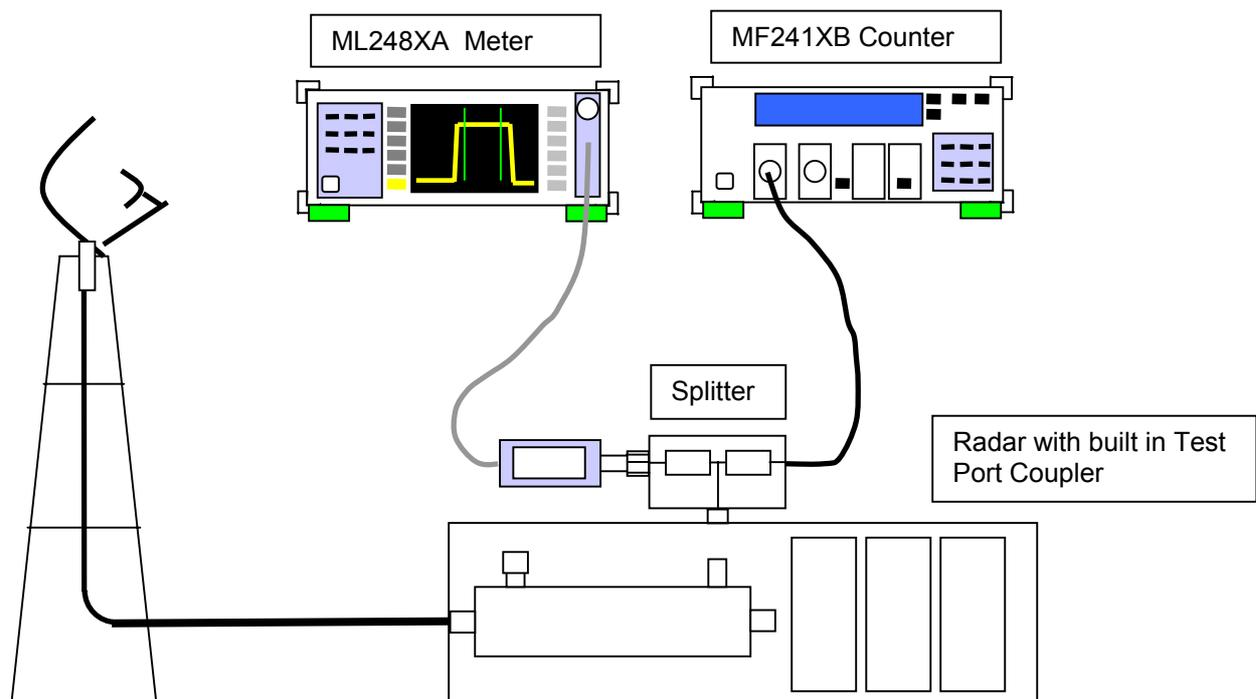
Figure 1. Typical Pulse Radar Measurement Set Up
