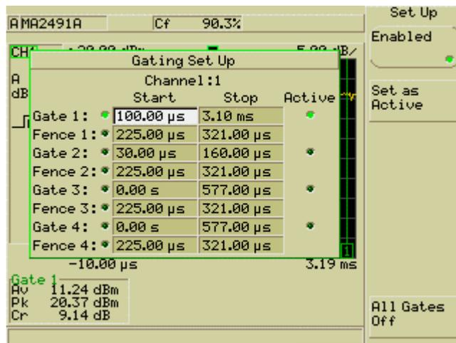
Figure 4. The Gating Set Up Dialog Box
