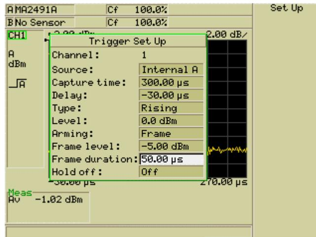
Figure 2. Trigger Set up Menu
