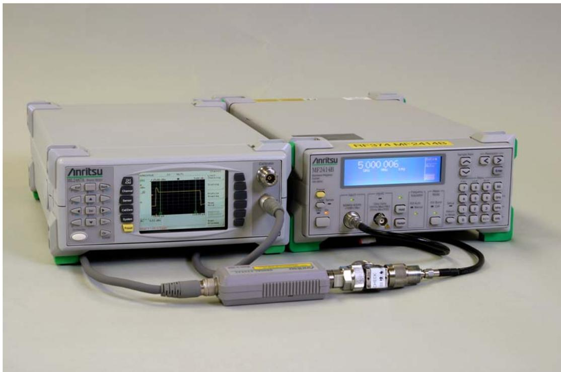
*Understand how to set up and use the Wideband Peak Power Meter and Frequency Counter for Radar measurements*
