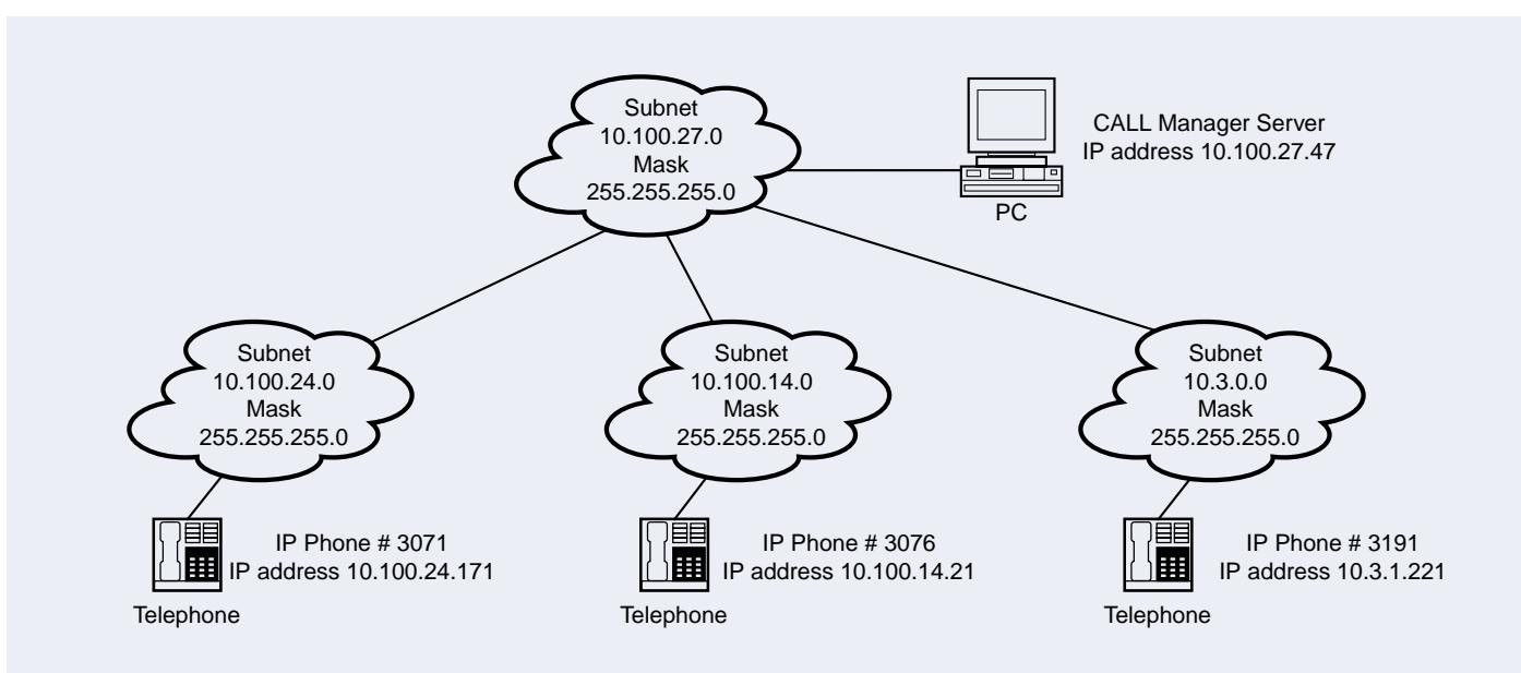
Figure 2: Network Subnet Configuration for IP Phone Evaluation
