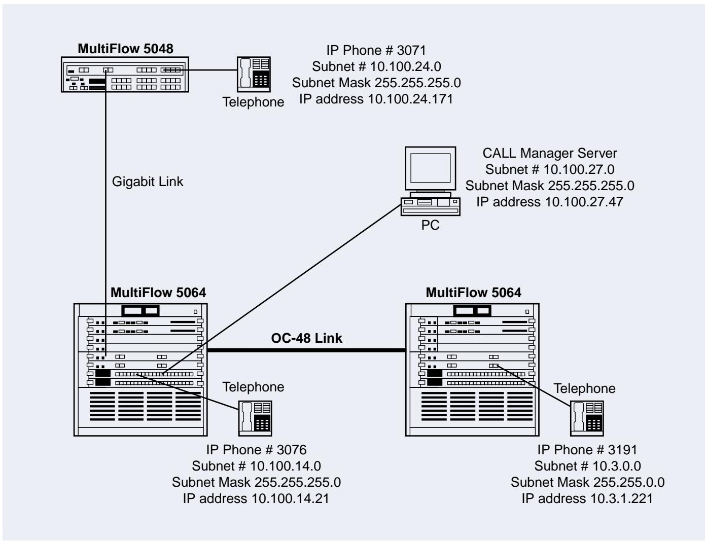
Figure 3: Network Physical Configuration for IP Phone Evaluation
