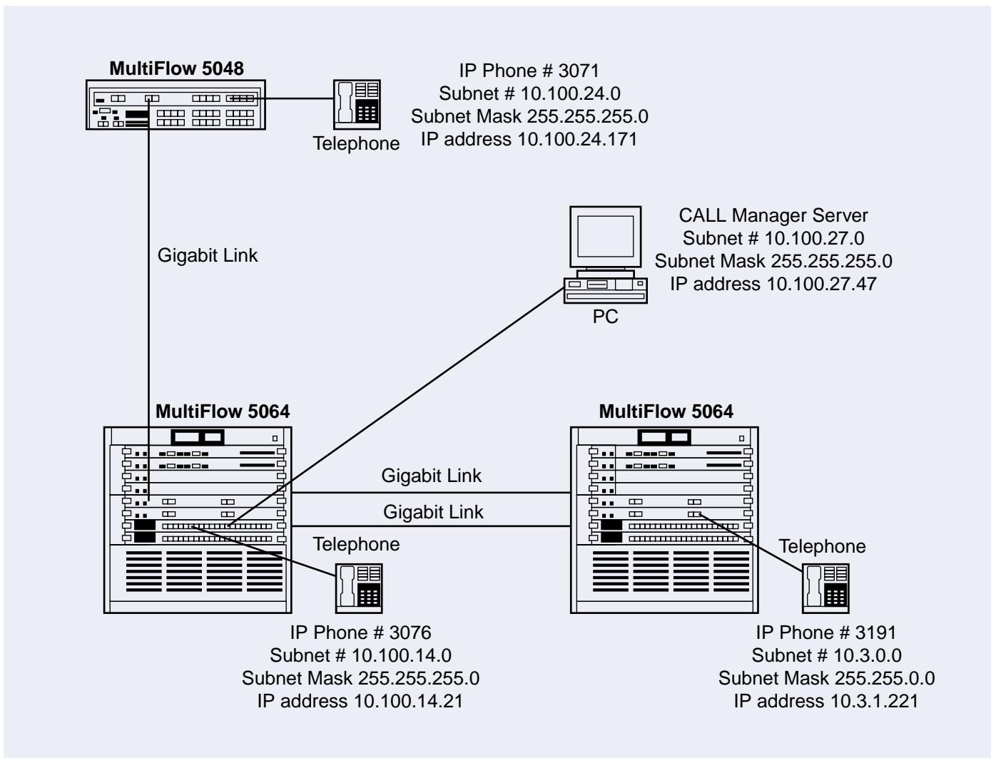
Figure 5: Configuration for Fault Tolerance Evaluation by Link Aggregation
