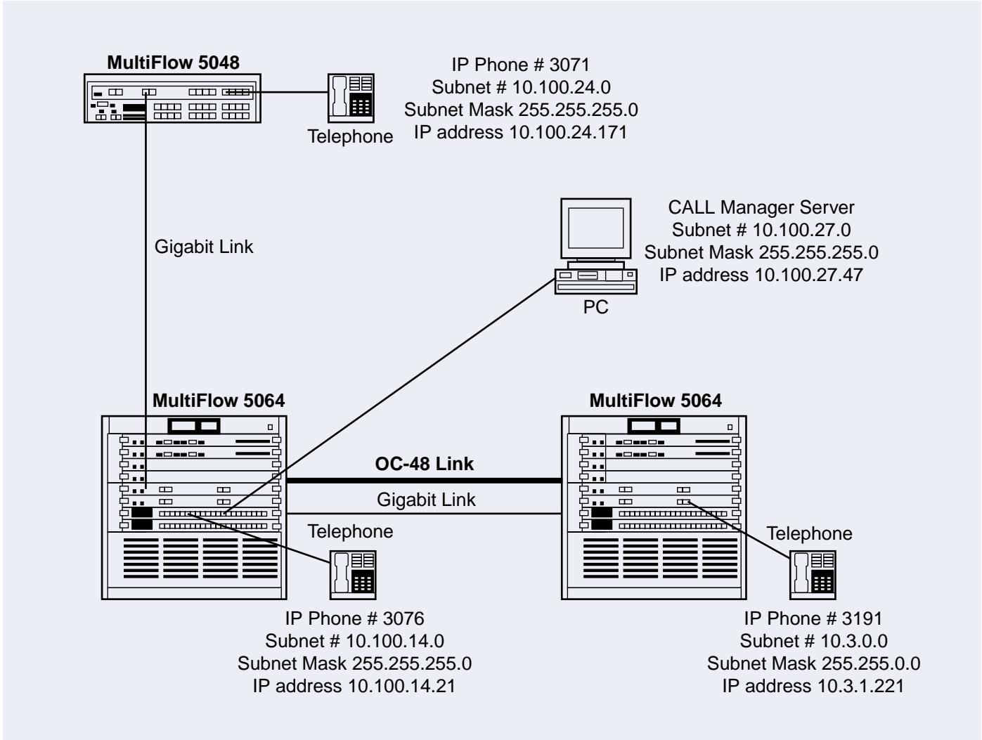
Figure 4: Configuration for Fault Tolerance Evaluation by AQR
