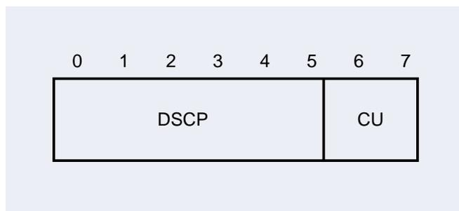
Figure 1: DS Field Structure
