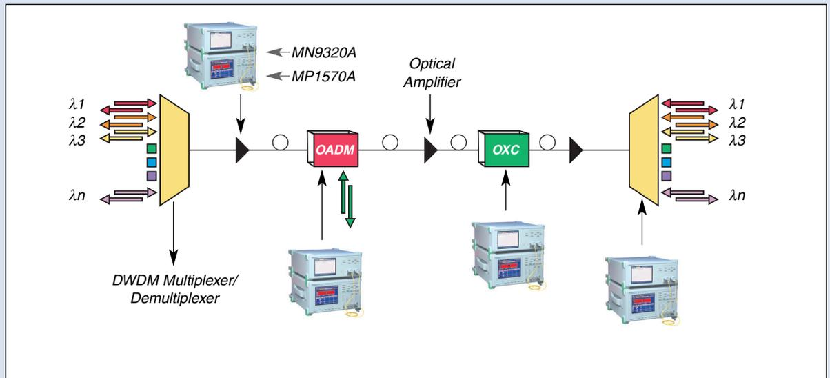
Dense Wavelength Division Multiplexing (DWDM), is a technique used in fiber optic transmission to expand the traffic carrying capacity of a single fiber. It has been widely adopted by network operators globally as a means of increasing the capacity of their existing networks without the need for additional and very costly re-cabling. DWDM expands the design possibilities for an All Optical Network (AON), based on its channel add and drop functionality.
