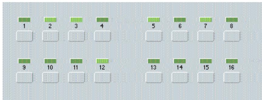
During a measurement, the MP176x tests bit 1 first, then bit 2, etc. During setup, the bits within each page are transmitted from the computer to the instrument over GPIB in the opposite order from the display; i.e., bit 16 is sent first, followed by bit 15 and so forth. The overall sequence of pages is unchanged; in other words, page 0 is sent before page 1.
