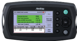
MT9090A with MU909011A Mainframe with Fault Locator Module
