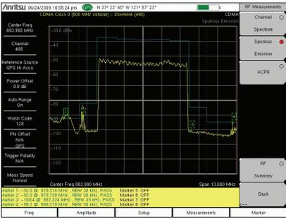
**RF Measurements – Spectral Emissions Mask**
