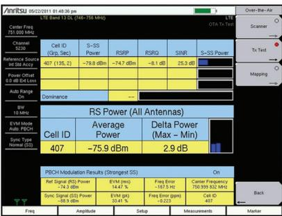
**Over-the-Air Measurements - Tx Test**
