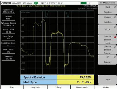
**RF Measurements – Spectral Emissions Mask**
