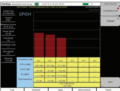
**Over-the-Air Measurements – Scrambling Codes**
