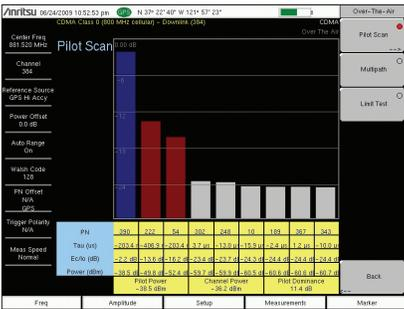
**Over-the-Air Measurements – Pilot Scan**
