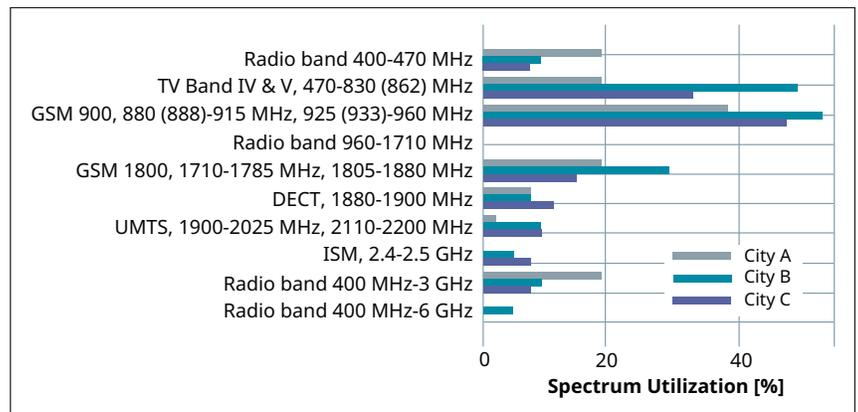
Figure 10. Spectrum Occupancy Measurement
