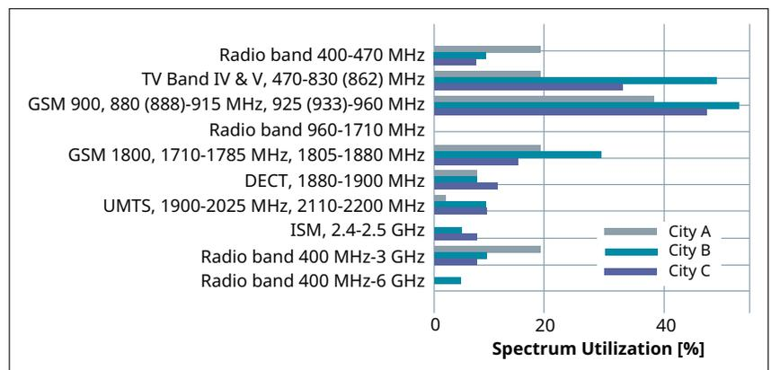
Figure 10. Spectrum Occupancy Measurement
