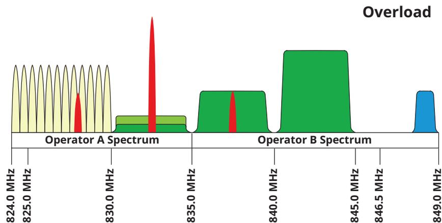
Figure 2. Malfunctioning Repeaters May Block Cellular Transmissions
