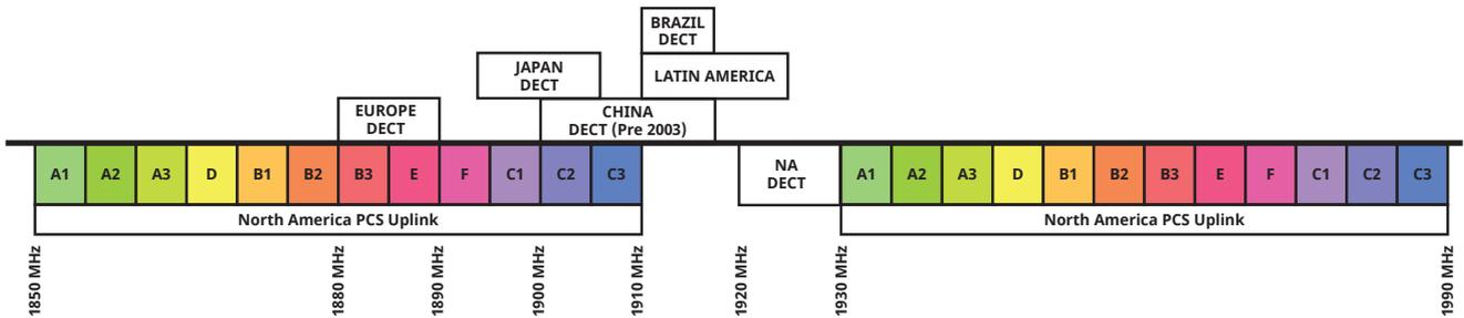
Figure 10. DECT Phones Improperly Used Can Cause Unintentional Interference
