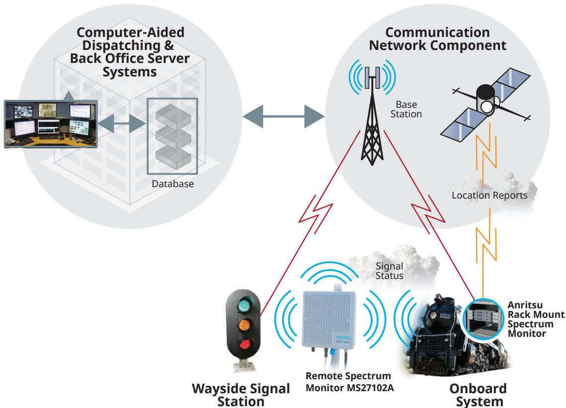
Figure 1. Spectrum Monitoring System Monitoring PTC Frequencies
