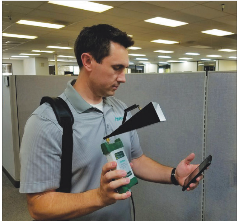
Figure 4. Millimeter-wave Indoor Coverage Mapping Solution
