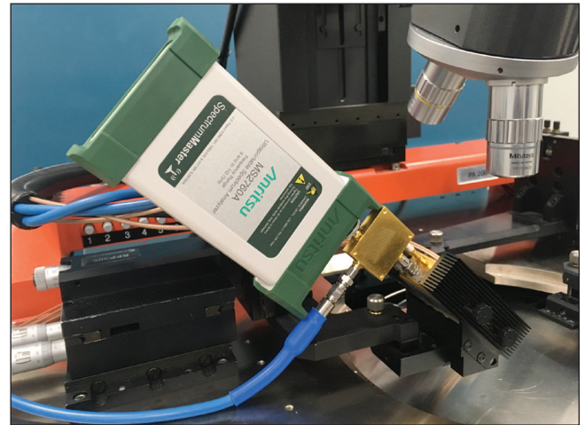
Figure 5. The Spectrum Master MS276xA is Connected Close to the Probe Tip on a Wafer Probe Station.
