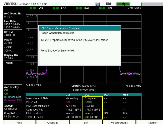
Automatic reporting capabilities cycle through all ULs tested, gathering all JPGs and measurement files generated
