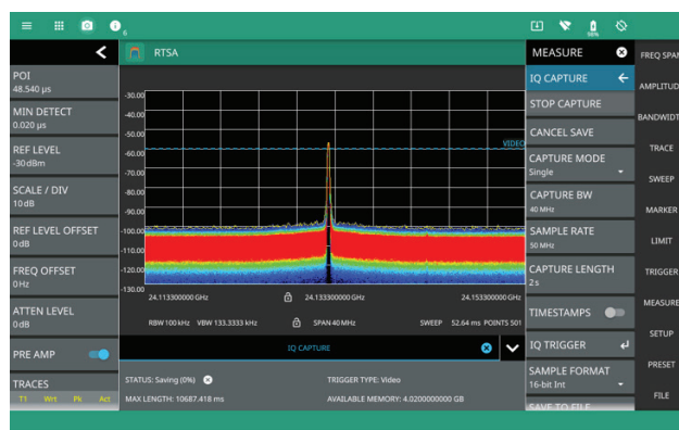
Free Run, External, Video, and Level Trigger Options are Available in the RTSA Mode to Initiate IQ Data Capture
