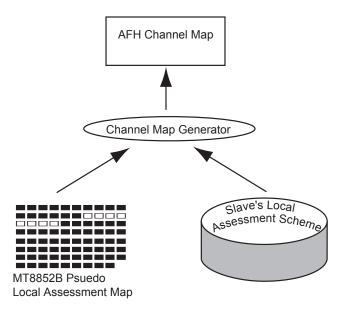
The Active Channel Map defines the permitted channels that the MT8852B and EUT use whilst frequency hopping.
