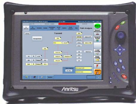
The compact size of the XTA Application module conveniently fits into the CMA 5000 Multi-Layer Network Test Platform using a small bay adapter - thus reducing cost and overall weight.
