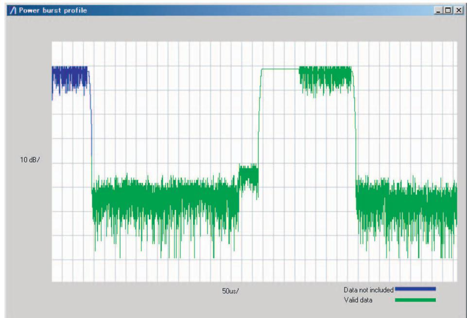
*Example profile of a 2-DH1 EDR packet*
