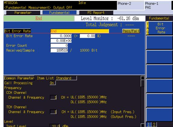
Bit error rate measurement (8PSK)
