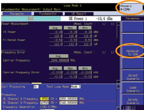
W-CDMA Measurement (Test loop mode or voice communications)
