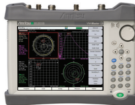
MS2034B/MS2035B 500 kHz to 4 GHz/6 GHz 100 kHz to 4 GHz/6 GHz Vector Network Analyzer with Spectrum Analyzer
