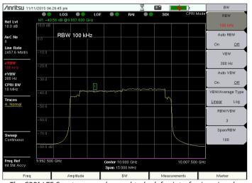
The CPRI LTE Spectrum can be used to look for interferring signals on the uplink and can also be used to verified the downlink BBU
