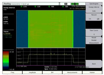
The CPRI RF Spectrogram can be used to find intermittent interferers over a period of time.
