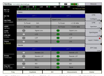
The BTS Master displays CPRI alarms which helps verify CPRI link status.
