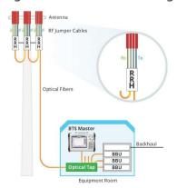
Anritsu's CPRI testers display LTE uplink or downlink spectrum by tapping into the fiber between the BBU and RRH.
