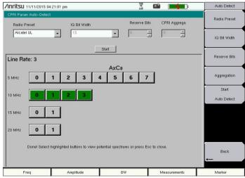
CPRI Auto detect allows users to choose radio preset which determines line rate, signal bandwidth and AxC.
