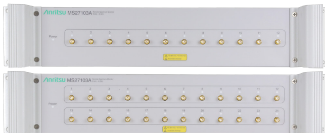
The MS27103A is housed in a rack-mountable enclosure with 12 (or optionally) 24 RF Inputs. An electronic switch is used to address each port. The MS27103A is a full featured platform for monitoring and recording signals at user specified frequencies.
