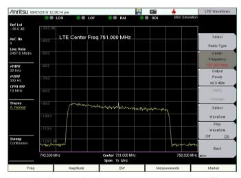
In BBU Emulation mode BTS Master can stream an LTE wavefile to the RRH that is transmitted at maximum power in the downlink. At the same time it can display the LTE uplink spectrum, monitoring for interfering signals or the presence of PIM.
