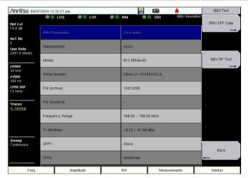
After initializing the remote radio head, the BTS Master displays CPRI Layer 2 status alarms and the full configuration of the RRH.
