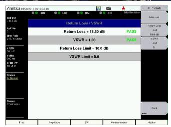
The return loss and VSWR at the remote radio head transmit port can be read over the CPRI link and displayed with pass/fail status on the BTS Master display.
