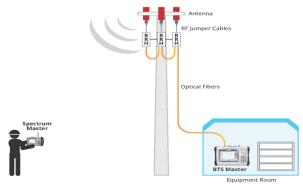
Using a second Anritsu spectrum Analyzer, the LTE wave file transmitted on the RRH downlink can be viewed.
