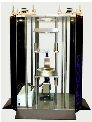
Open Resonator Method (DPS 03) for Sheet and Ultra-Thin Sheet
