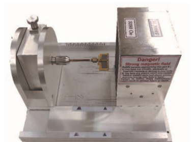
Magnetic Property Characteristics (Including Magnetic Permeability) Measurement System
