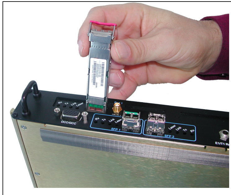
Fig.4: Change the optical interface of your module in the field via XFP transceiver
