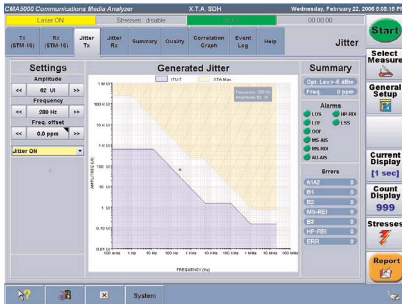
Graphical display of the generated jitter (frequency and amplitude) compared to the recommended maximum tolerable jitter mask of the equipment under test
