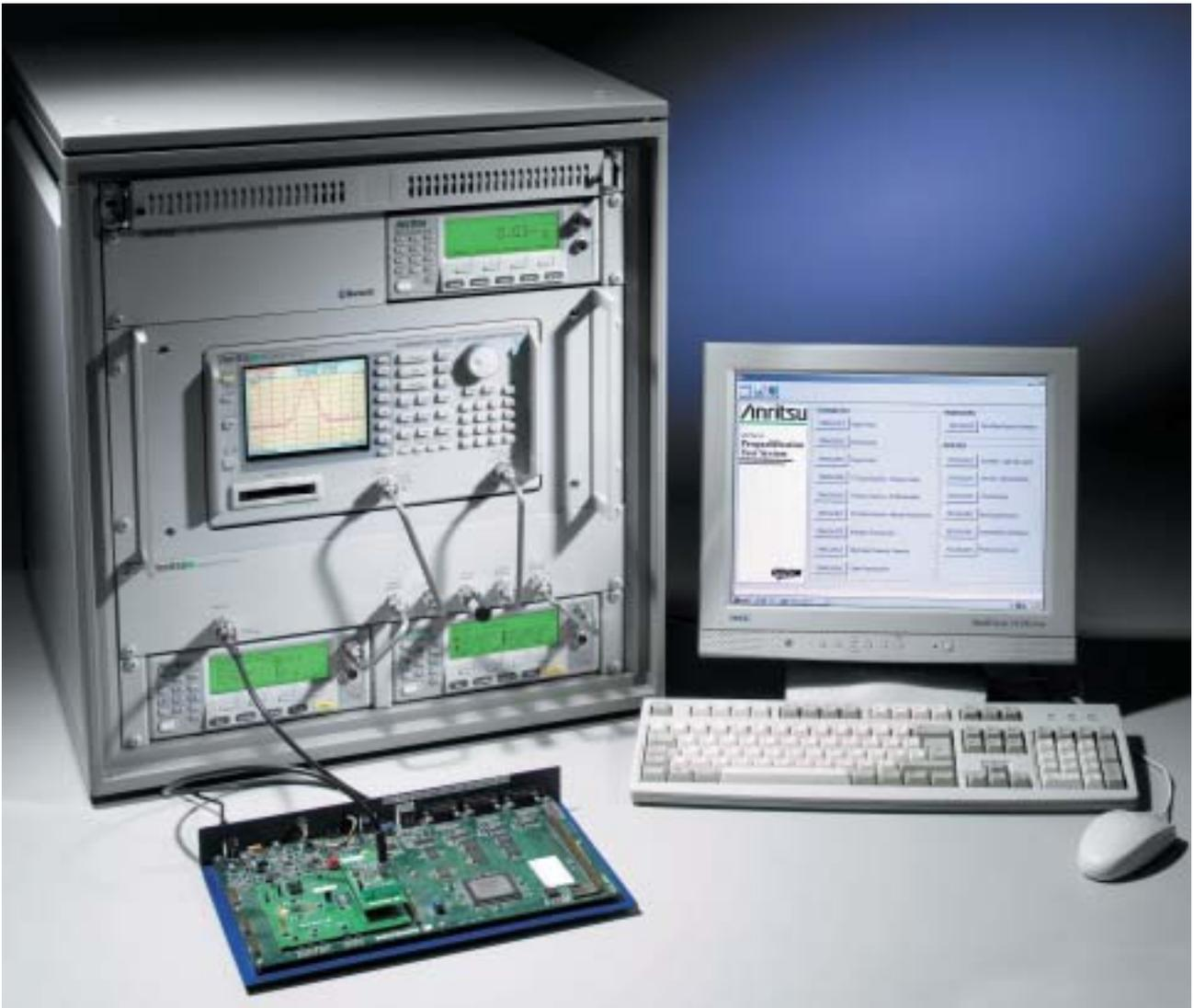
*Perform measurements on Bluetooth radios according to the RF Test Specification*
