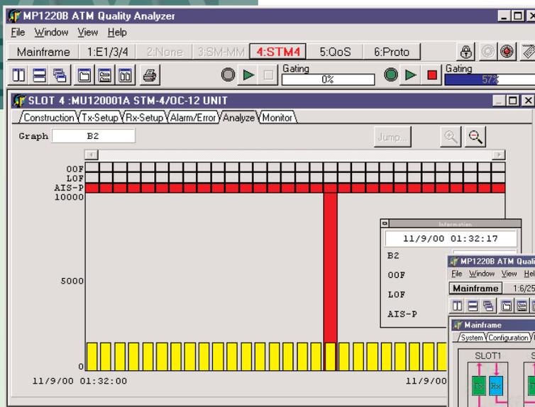
Injecting and monitoring for error or alarm status of an optical network can be done using the STM4 option unit.
