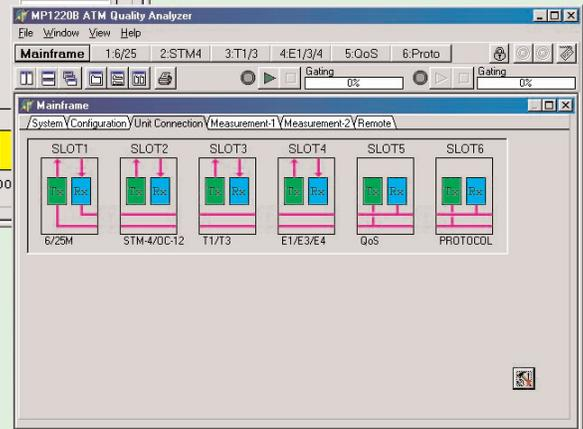
ATMQA<sup>®</sup> mainframe configuration software defines the flow of data across the option units contained in the mainframe chassis.
