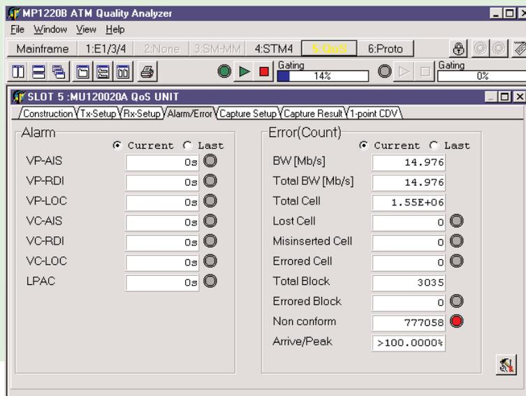
*Non-conforming ATM Cell which exceed the bandwidth allocation of the GCR Algorithm can be detected by the MP1220B.*
