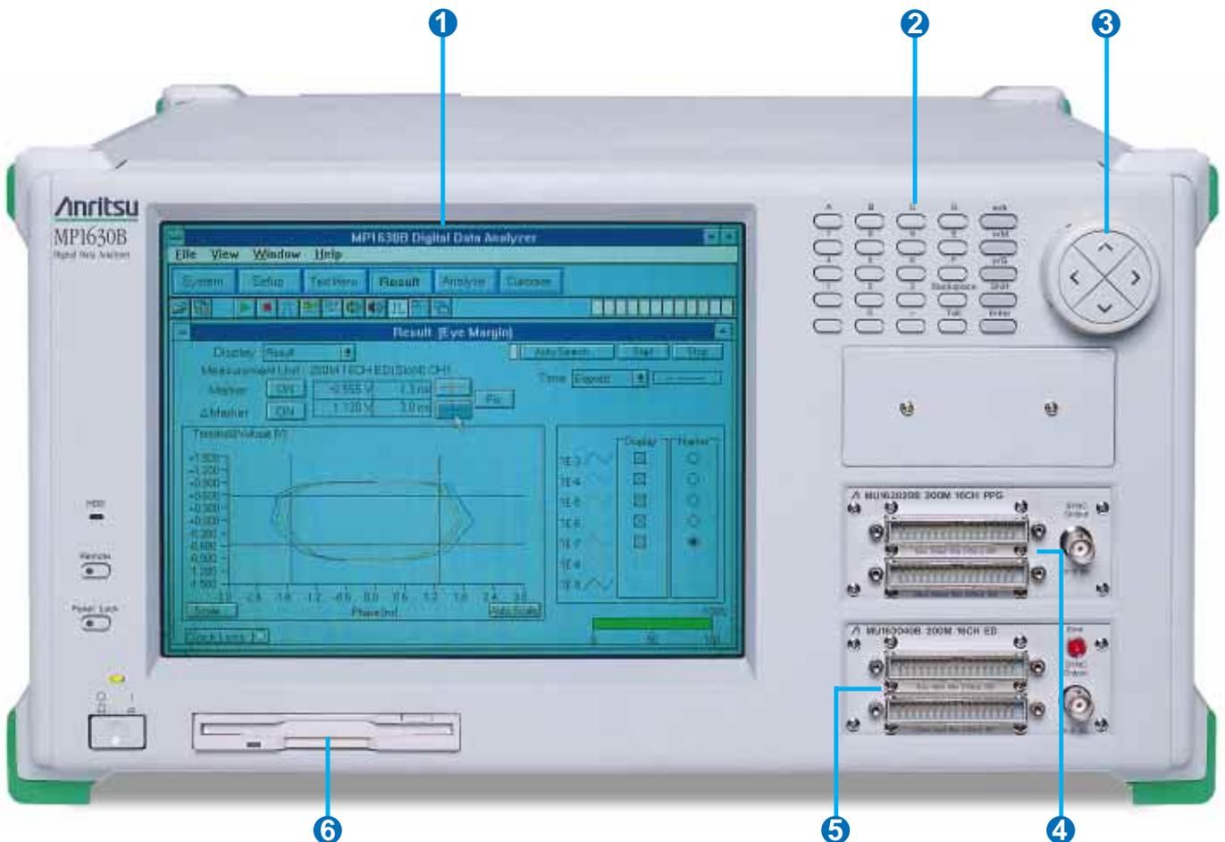
**4 Pulse Pattern Generator Unit (200 Mb/s, 16 channels)**
