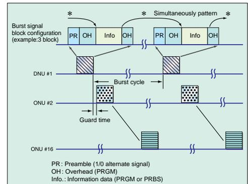
Example of burst data output for PON module test
