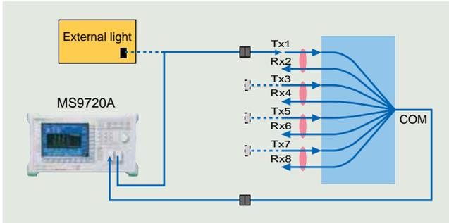
By using the same setup, it is possible to measure the optical leakage between each channel of an optical coupler and to measure the isolation. Moreover, when used in combination with an external light source, it is possible to measure the directivity to evaluate the very weak optical leakage between send and receive channels.
