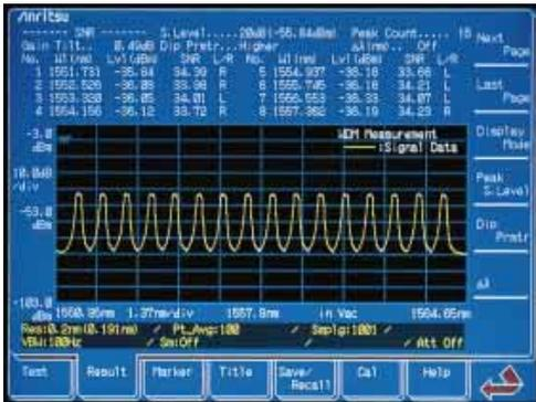
The screen below shows analysis of a 16-channel WDM waveform; the level difference of each channel is displayed using the channel on the left side as a reference. Any channel can be set as the reference.
