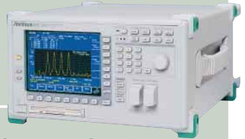
The MS9720A is an optical spectrum analyzer with a diffraction grating that is used to measure and analyze optical spectra in the 1450 to 1650 nm band for WDM communications systems.
