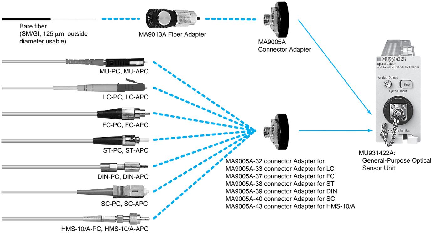
● **Applicable fiber : GI/SM** (9/125 to 62.5/125  $\mu\text{m}$ , NA:  $\leq 0.29$ )
