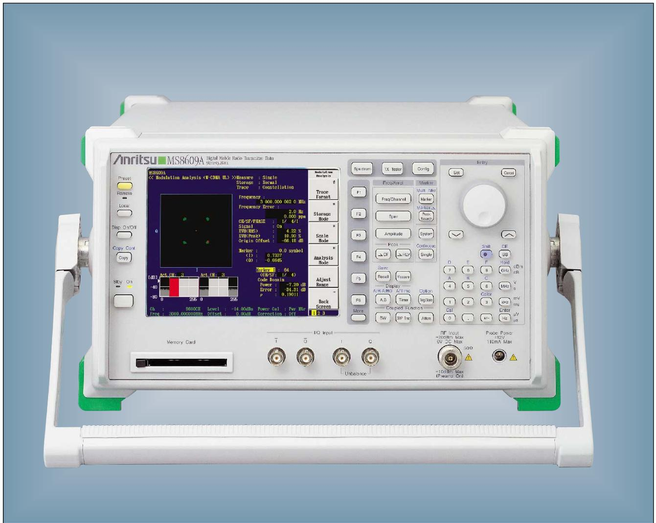
*For Transmit Modulation Analysis Evaluation of W-CDMA Mobile Terminals*
