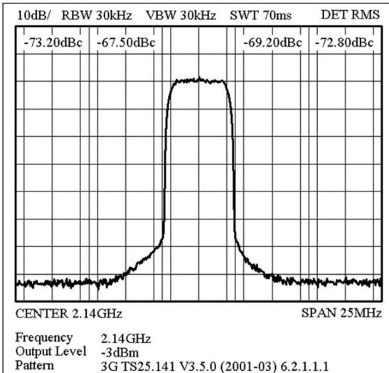
Adjacent channel leakage power ratio at 16 channel multiplex
