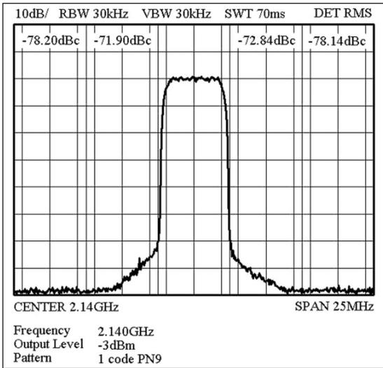
Adjacent channel leakage power ratio at 1 channel
