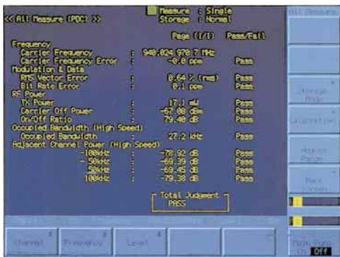
In addition to defining limit value for pass/fail decisions, the user can also specify whether pass/fail decisions are to be made and define the measurement items and methods.
