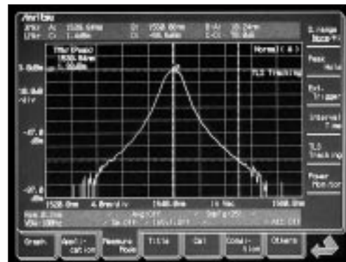
B: Wide dynamic range measurement (MS9710B display)
