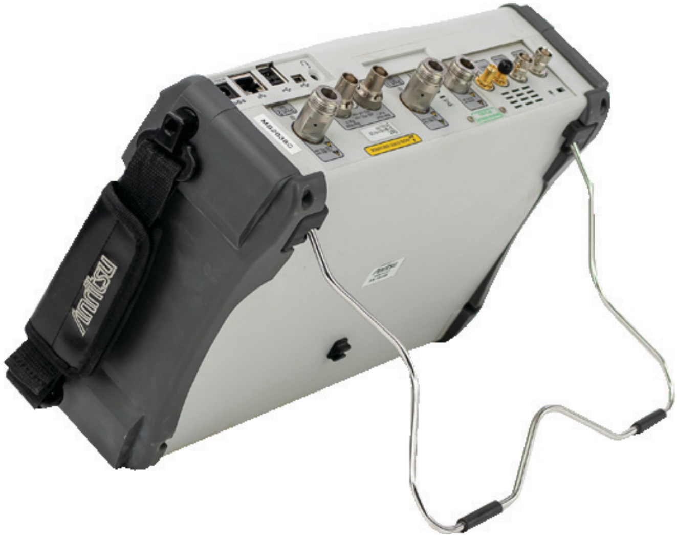
Figure 1-1. Wire Tilt Bail on Thick Cased Instrument
