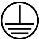
The MS27102A chassis provides two earth ground connections. Be sure to ground the instrument chassis and any antenna installations in accordance with your local regulatory requirements. Failure to properly ground the equipment may present an electric shock hazard and contribute to static noise interference.
