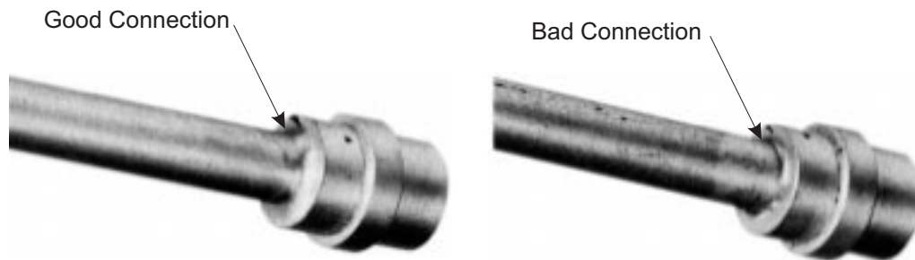
Figure 3-4. Examples of Good and Bad Solder Connections
