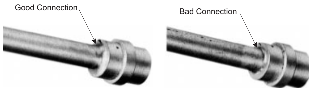
Figure 2-4. Examples of Good and Bad Solder Connections
