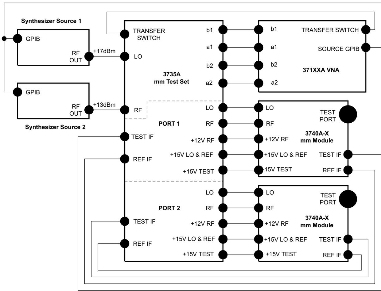
Figure E-3. 371XXA Millimeter Wave VNA System Interconnections
