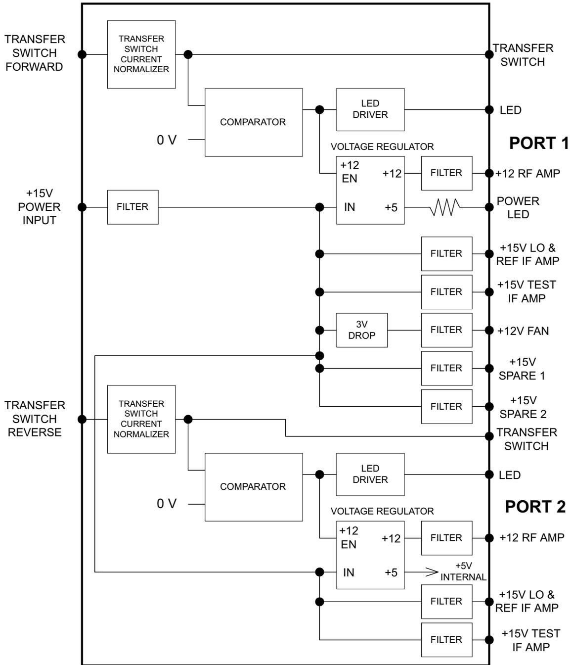
**Figure E-5.** 3735B Test Set PCB Assembly Block Diagram
