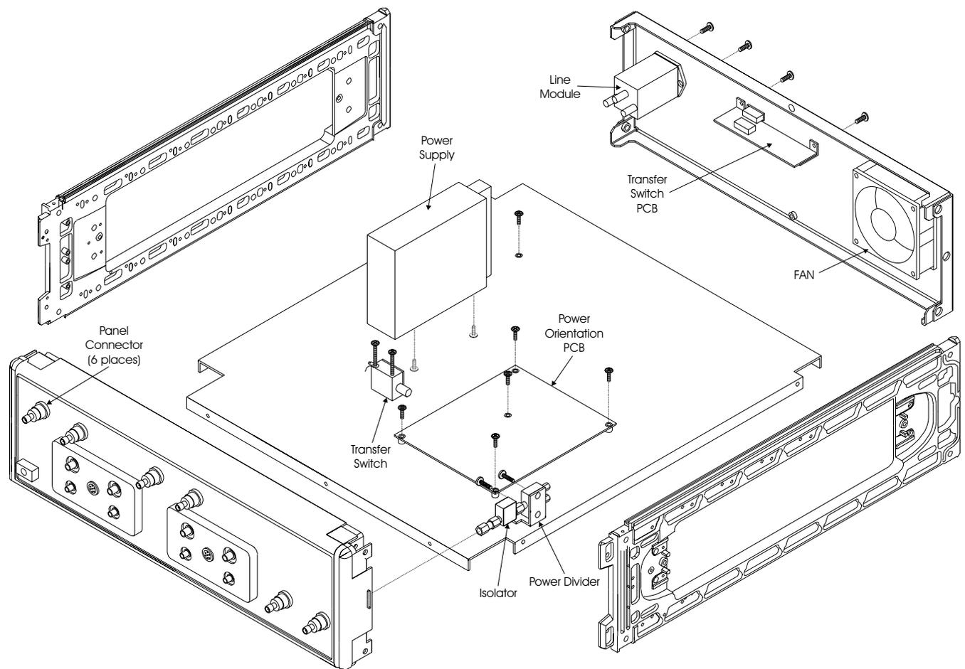
**Figure E-8.** *Replaceable Parts Exploded View*
