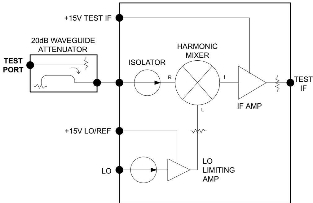
**Figure E-7.** 3741A-X Millimeter Wave Module Block Diagram
