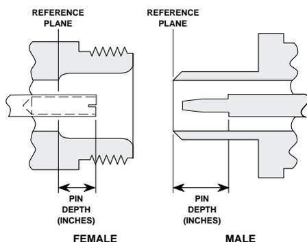
Based on ANRITSU precision components returned for repair, destructive pin depth of mating connectors is the major cause of failure in the field. When a precision component is mated with a connector having a destructive pin depth, damage will likely occur to the precision component's connector. A connector is considered to have destructive pin depth when the center pin is too long in respect to the connector's reference plane (Figure C-1).
