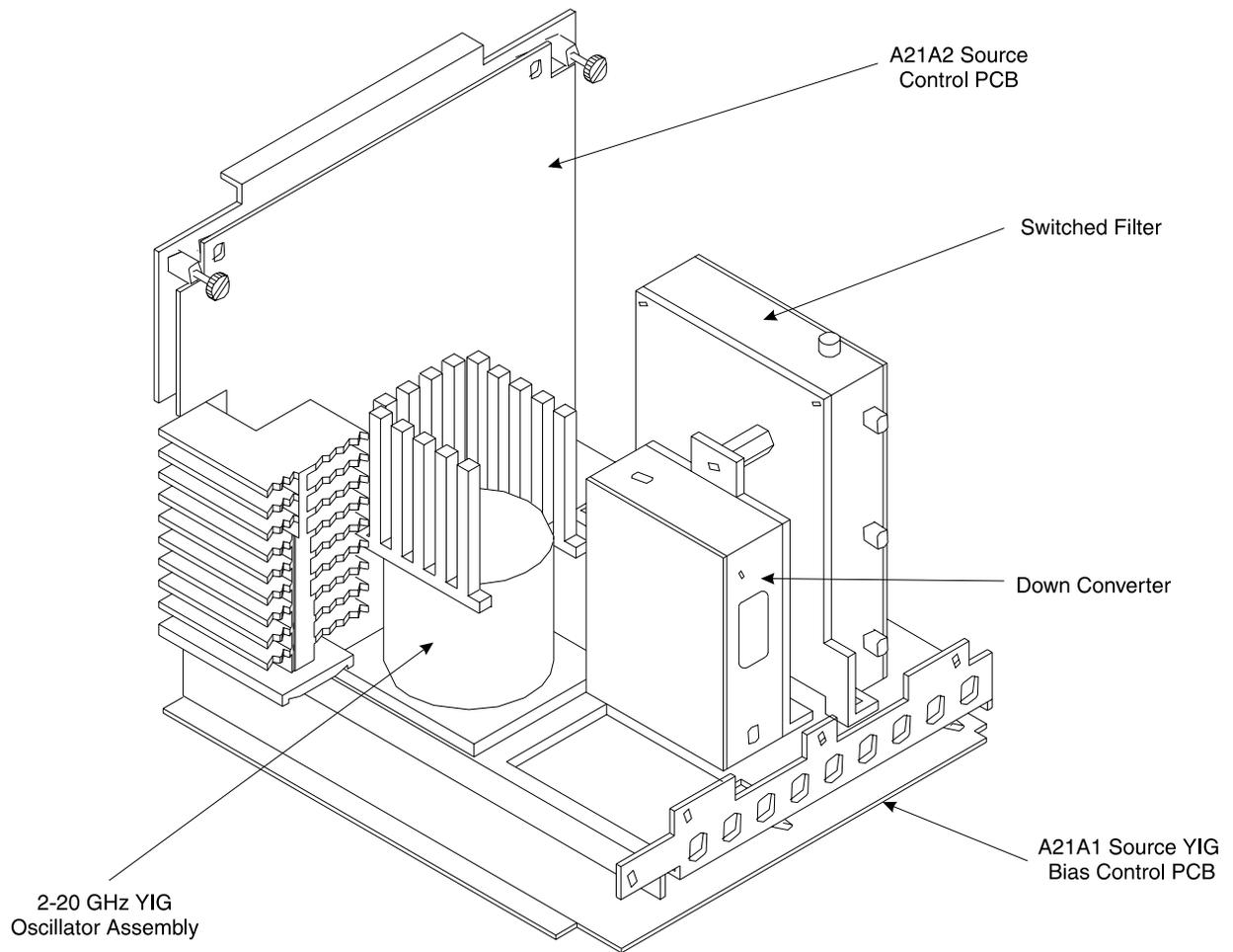
**Figure 2-3.** *Signal Source Parts Location Diagram*
