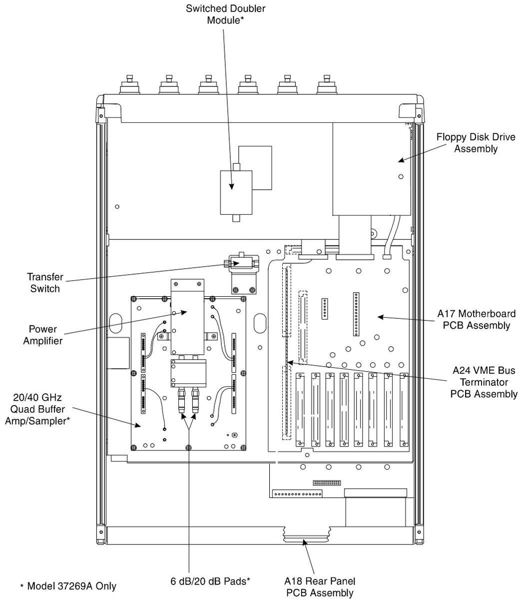
**Figure 2-2.** 371XXA Major Assemblies Location Diagram (Bottom View)
