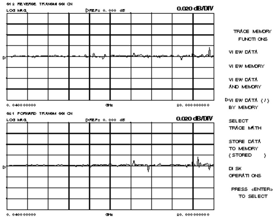
Figure 4-2. High Level Noise Test Waveform
