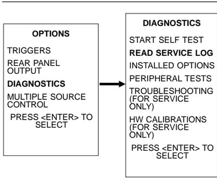
The 371XXA will now display the contents of the service log. The display consists of a header and an error listing. The header contains a variety of system service information. The error listing contains error messages for failures that may have occurred during operation.
