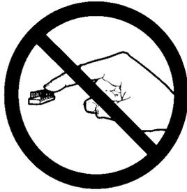
1. Do not touch exposed contacts on any static sensitive component.
