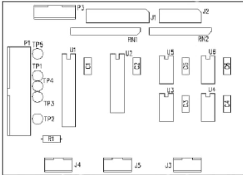
**Figure 4-6.** A6 Power Supply Parts Location Diagram
