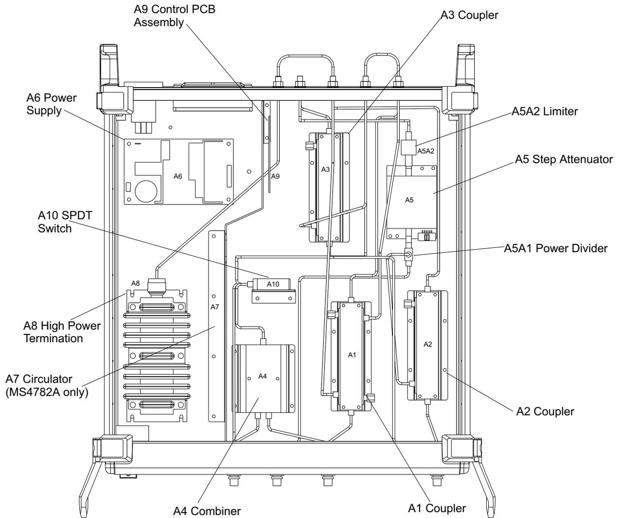
**Figure 2-1. Major Assemblies Location Diagram (Top View)**
