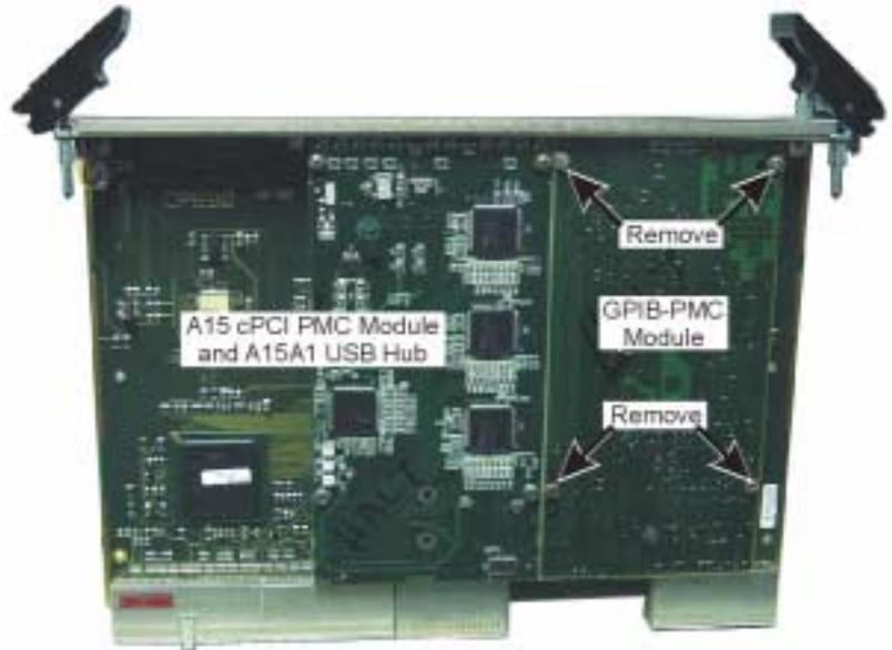
**Figure 6-36.** GPIB/USB Hub Module Removal
