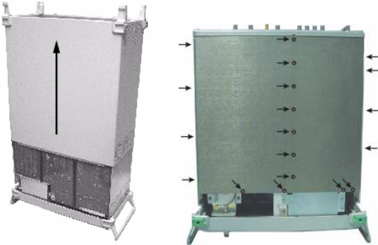
**Figure 6-2.** Chassis Cover Removal
