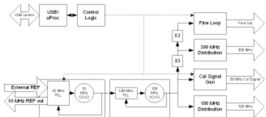
**Figure 1-5.** A6 Reference/Fine Loop Block Diagram
