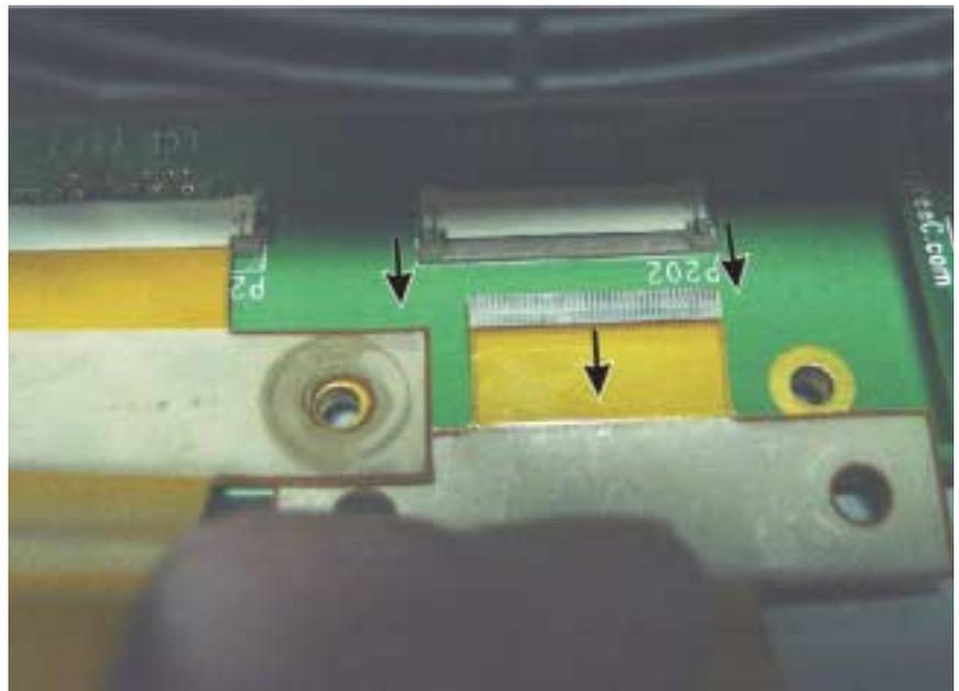
**Figure 6-10.** Front Panel Flex Circuit Removal
