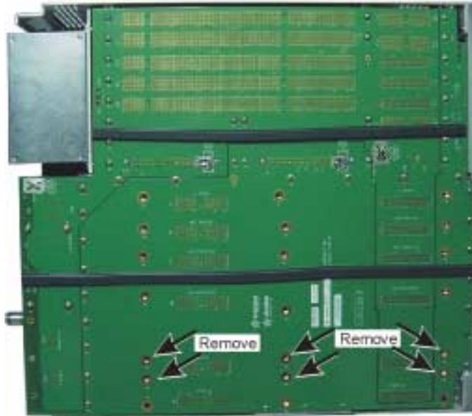
**Figure 6-11.** A3 Motherboard Screws
