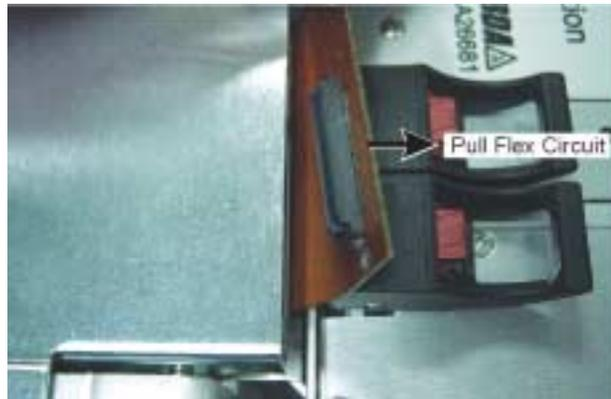
**Figure 6-52.** DVD Drive Flex Circuit Removal
