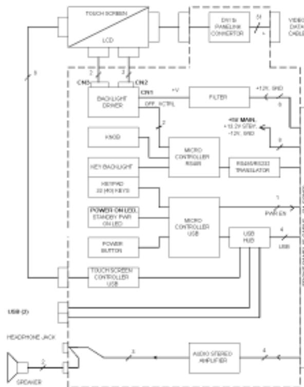
Figure 1-9. Front Panel Block Diagram
