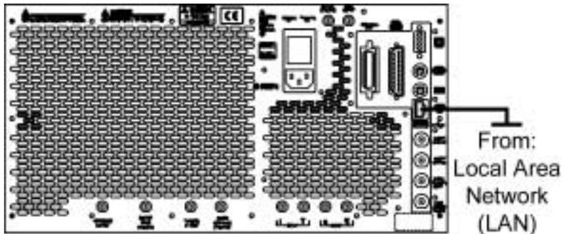
**Figure 2-17.** Ethernet Connection
