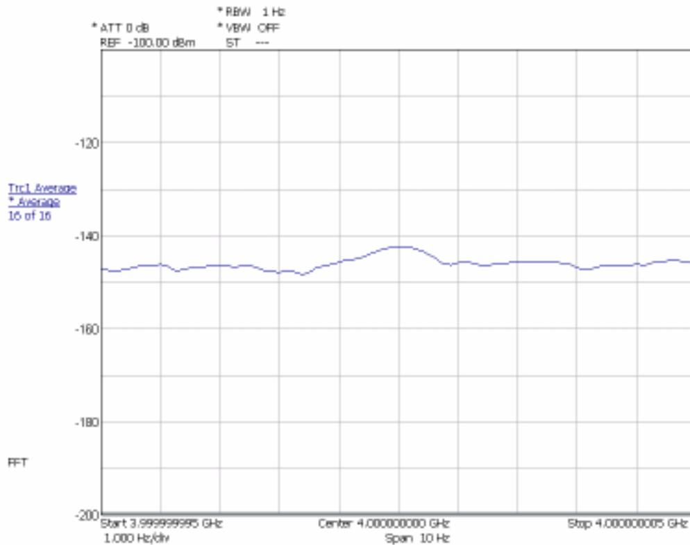
**Figure 3-7.** Displaying the Average Noise Level
