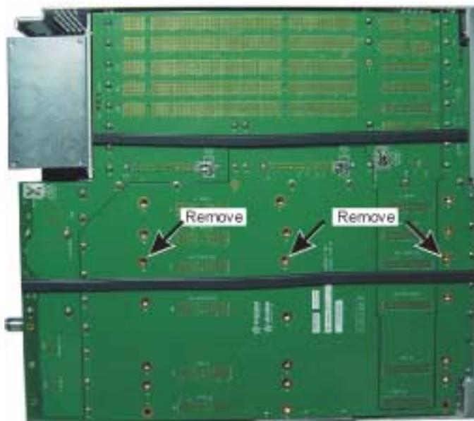
**Figure 6-18.** A5 Motherboard Screws
