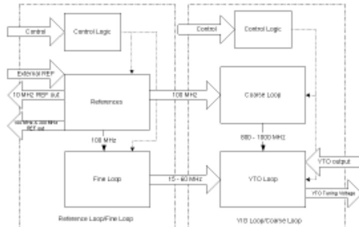
**Figure 1-4.** YTO Coarse Loop Module Block Diagram
