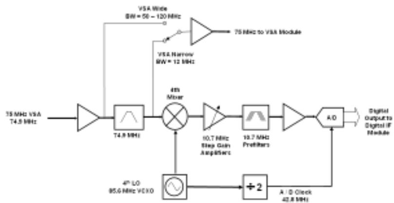
Figure 1-7. Output Section of A7 Analog IF Module
