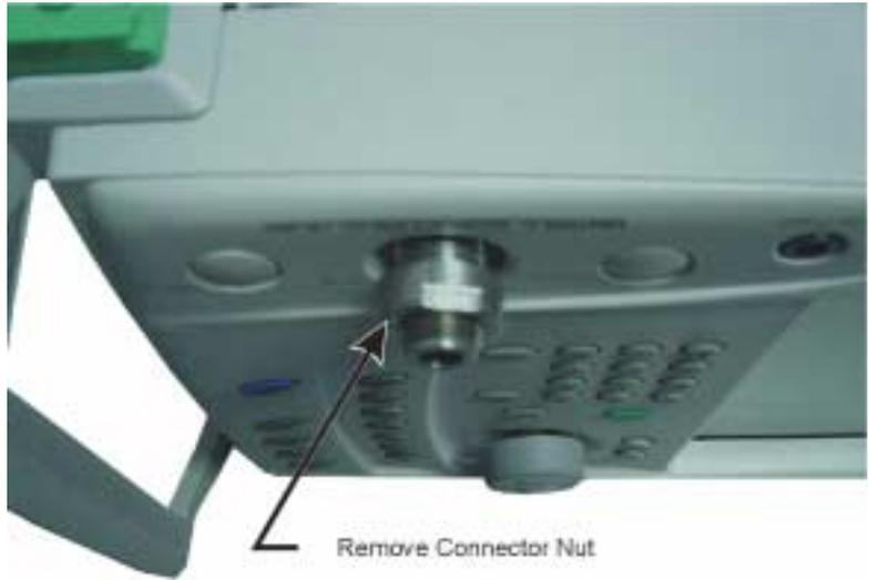
**Figure 6-5.** RF Connector Nut
