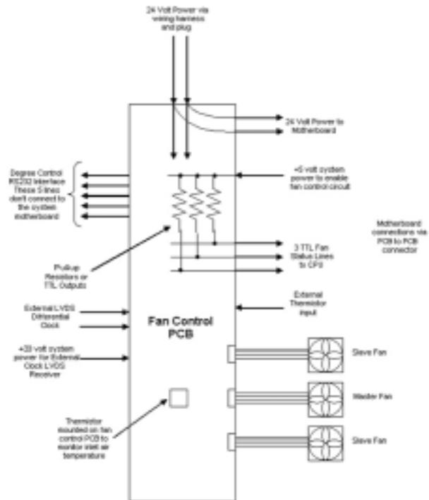
**Figure 1-8.** Fan Control Module Block Diagram
