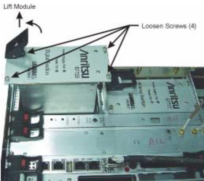
**Figure 6-27.** Digital Supply Removal
