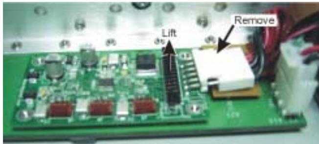
**Figure 6-46.** Fan Control Module Removal
