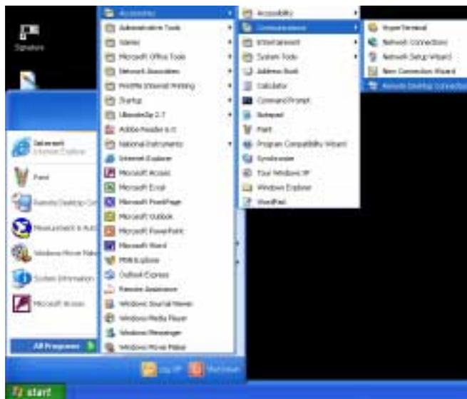
**Figure 5-8.** Starting a Remote Desktop Connection
