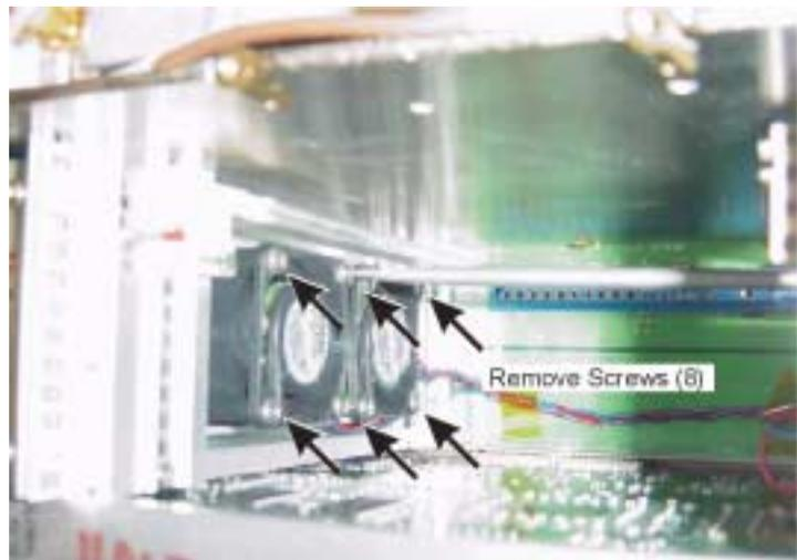
**Figure 6-57.** Removing Fan Screws
