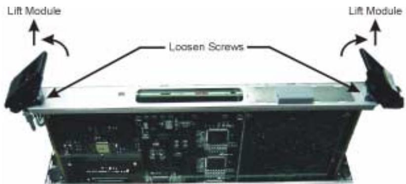
**Figure 6-35.** GPIB/USB Hub Removal
