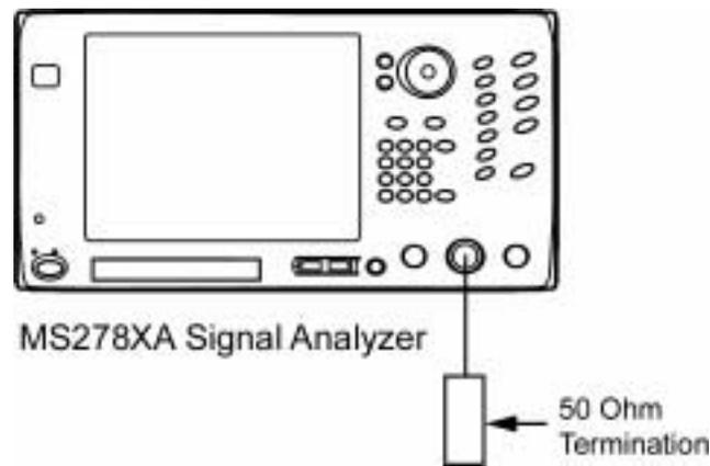
Figure 3-6. Equipment Setup for Average Noise Level Test
