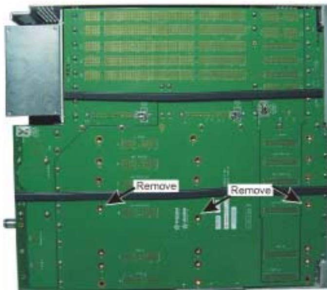
**Figure 6-15.** A4 Motherboard Screws
