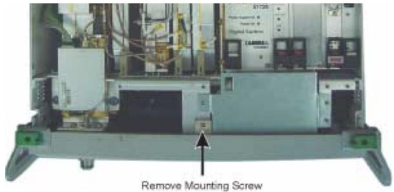
**Figure 6-6.** Front Panel Mounting
