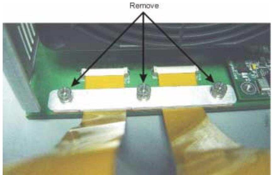
**Figure 6-9.** Front Panel Flex Circuit Strain Relief
