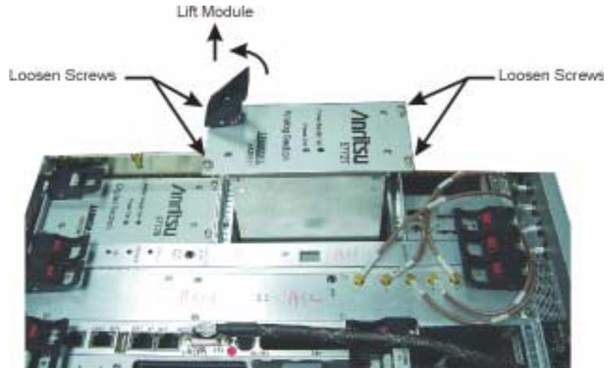
**Figure 6-26.** Analog Supply Removal
