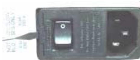
**Figure 6-58.** Opening the Rear Panel Fuse Cover
