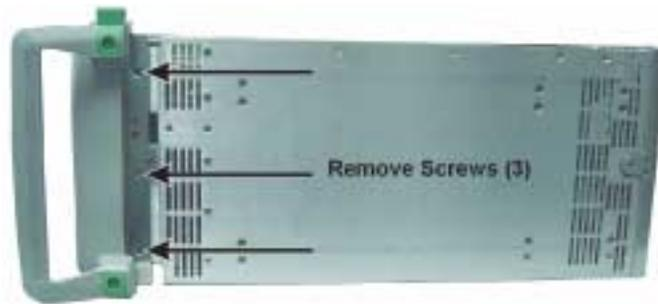
**Figure 6-7.** Front Panel Chassis Screws
