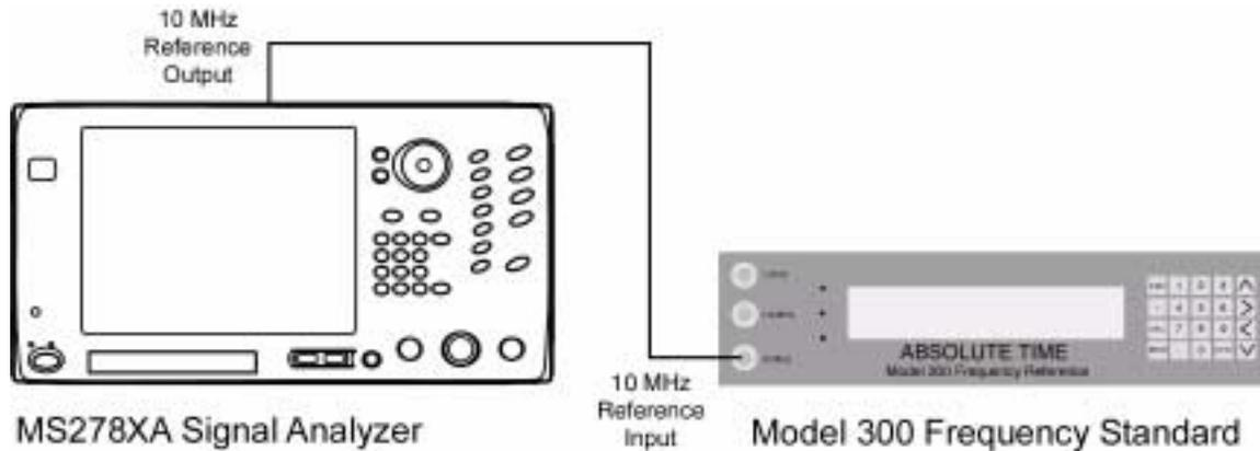
**Figure 3-1.** Equipment Setup for Internal Reference Oscillator Aging Rate Tests
