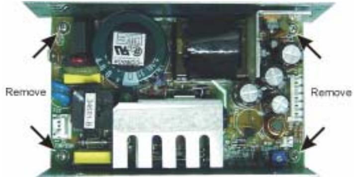
**Figure 6-49.** Standby Supply Removal
