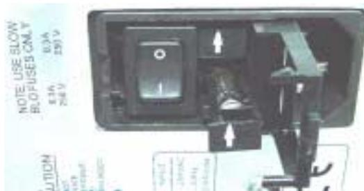
**Figure 1-11.** Replacing the Rear Panel Fuses
