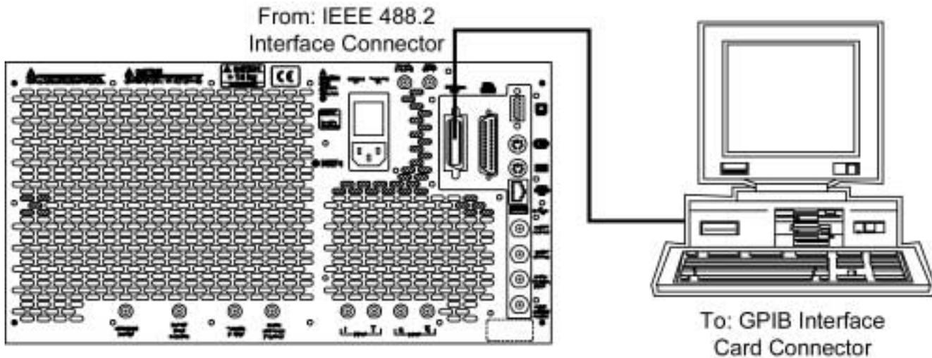
Figure 2-13. GPIB Setup
