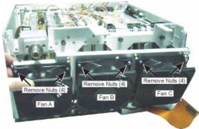
**Figure 6-44.** Fan Assembly Removal
