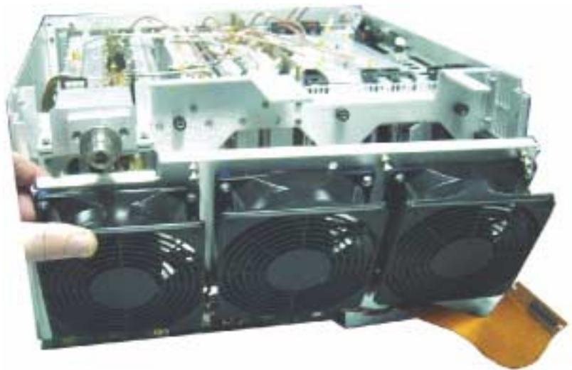
**Figure 6-43.** Fan Assembly Removal
