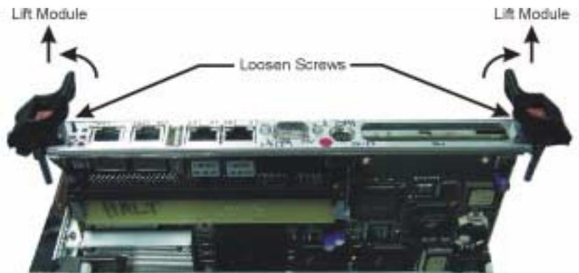
**Figure 6-33.** CPU Removal
