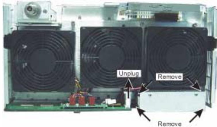
**Figure 6-47.** Standby Supply Removal
