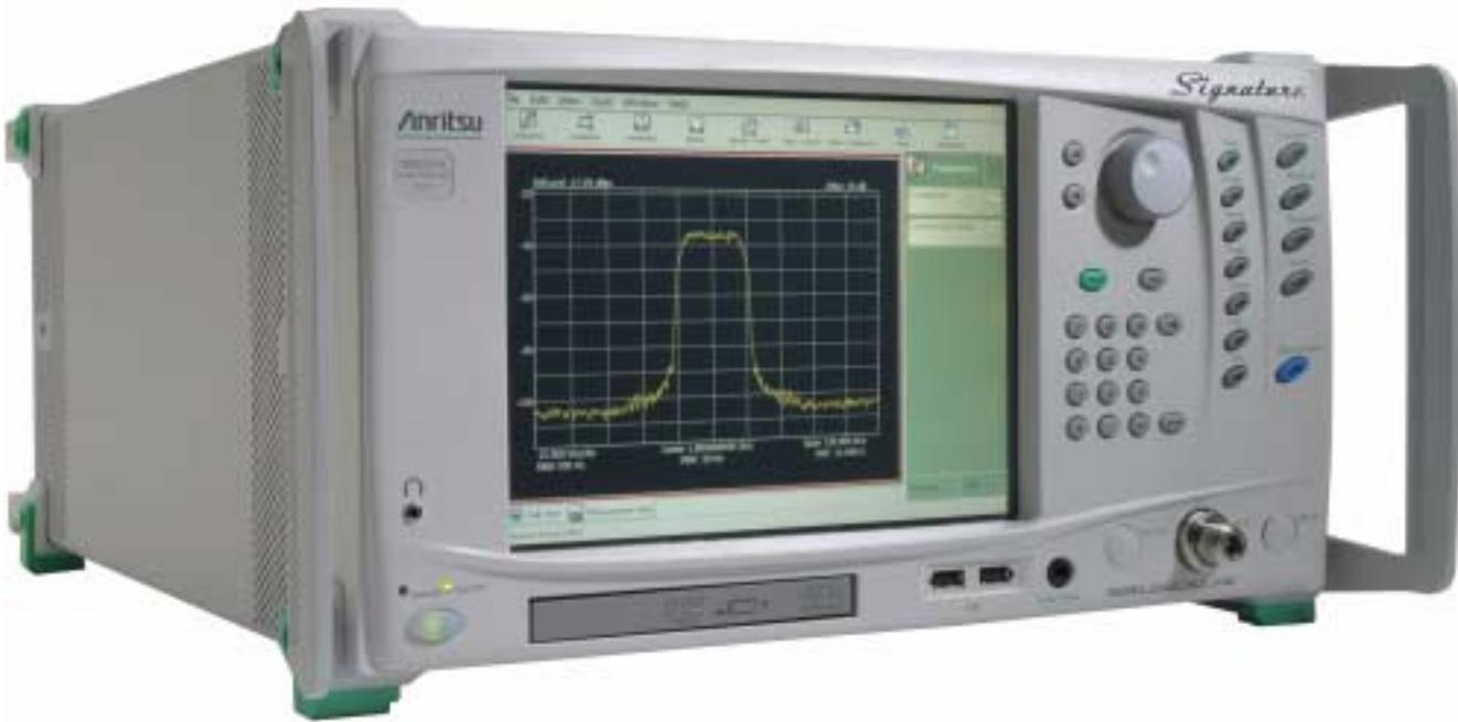
**Figure 1-1.** Signature Series MS278XA Signal Analyzer
