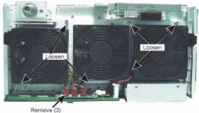
**Figure 6-42.** Fan Assembly Screws and Supply Leads
