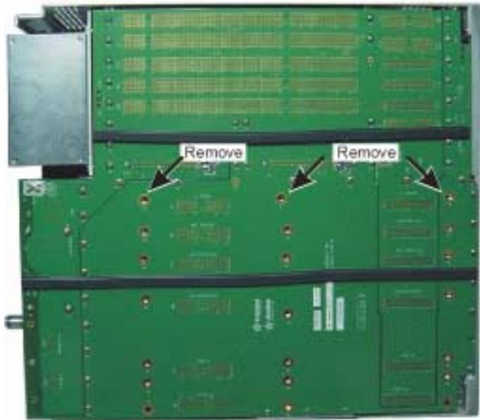
**Figure 6-24.** A7 Motherboard Screws
