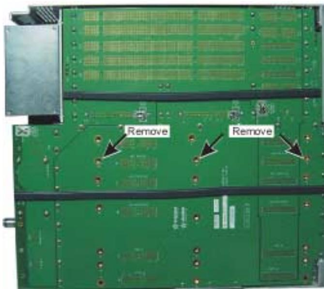
**Figure 6-21.** A6 Motherboard Screws
