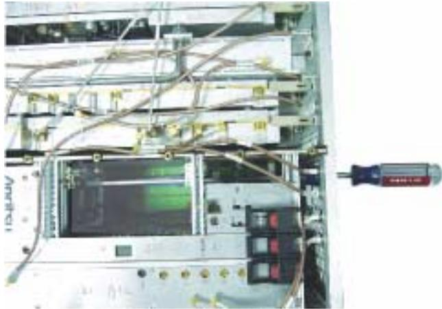
**Figure 6-56.** Power Supply Fan Removal
