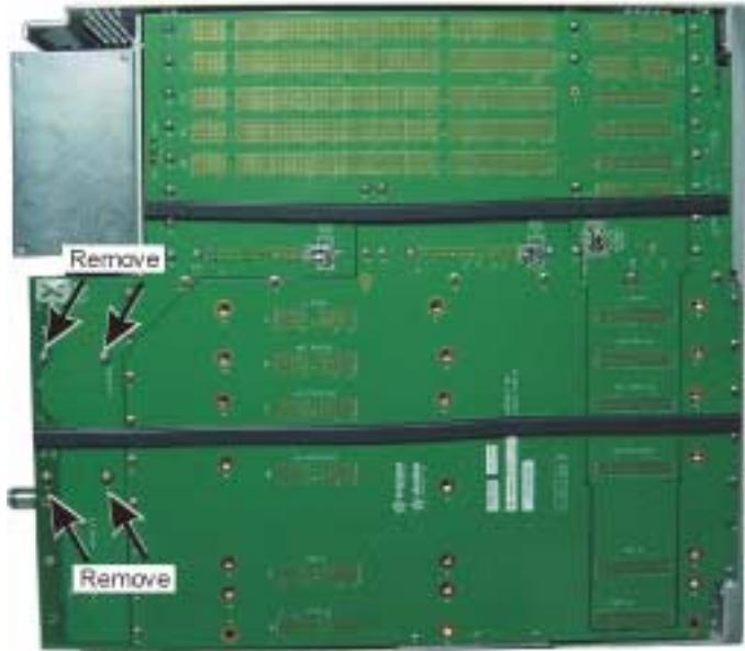
**Figure 6-45.** Fan Control Module Motherboard Screws
