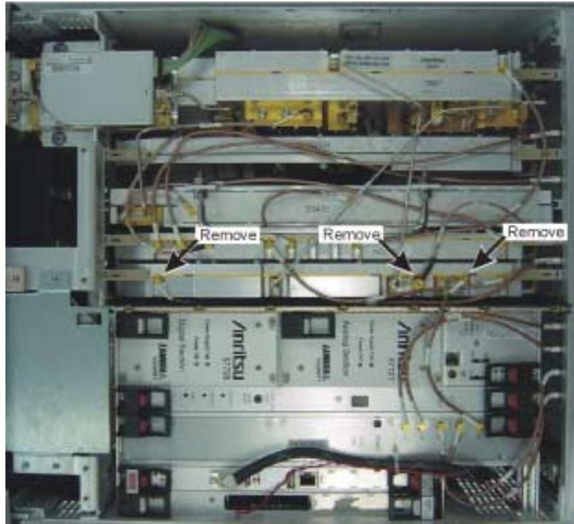
**Figure 6-23.** A7 Cables**Step 2.** Remove the RF deck as shown in “Removing the A3 RF Deck” on page 12.
