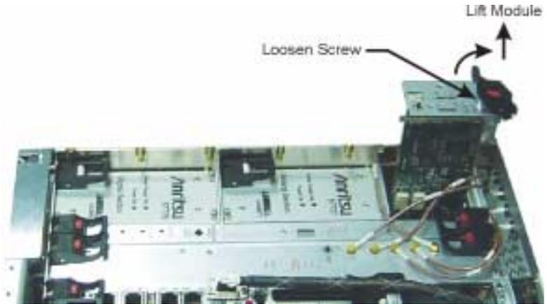
**Figure 6-37.** Chassis Control Module Removal
