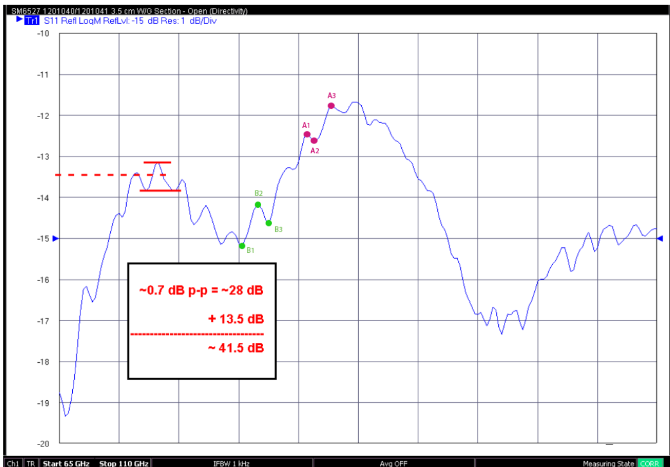
Figure 3-2. Markers Positioning for Directivity Verification
