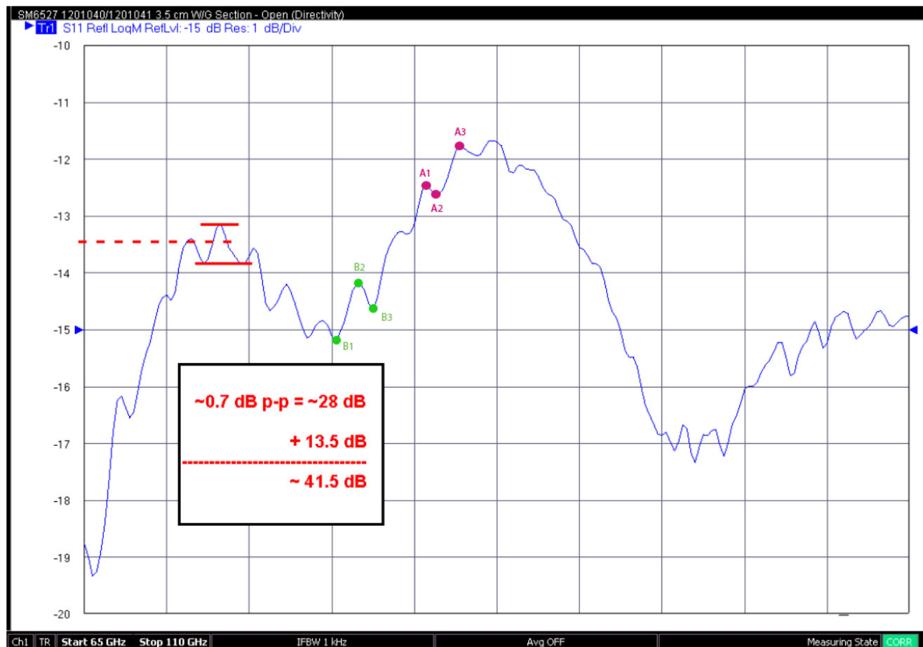
Figure 3-2. Markers Positioning for Directivity Verification
