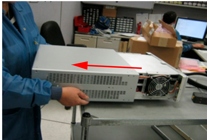
Figure 5-14. Manually Remove Chassis Cover
