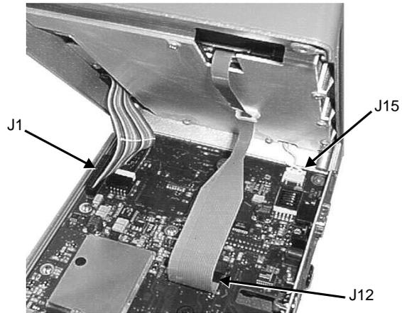
**Figure 11.** Spectrum Analyzer Front Panel Cable Connections
