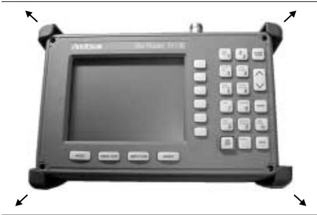
**Figure 12.** Removing the Corner Bumpers
