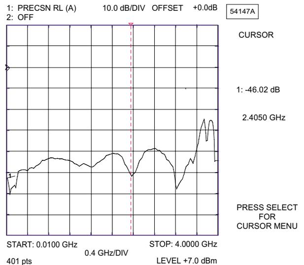
**Figure 6.** Direct Readout of the Precision Return Loss
