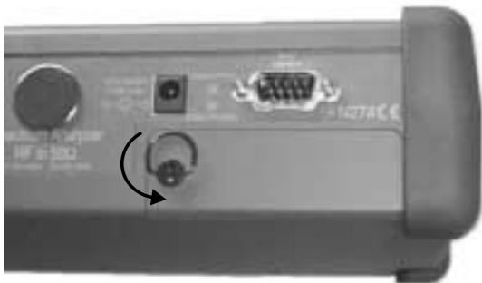
Figure 10. Rotate the Battery Access Door Handle
